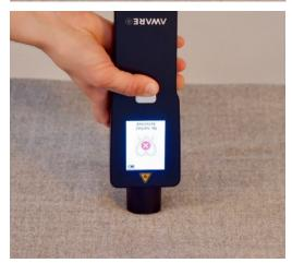
VIII. Turn off the lights of the room you're in. Put the garment on a flat surface to scan it. The hand scanner needs to touch the garment fully, without any gap in between. Move the scanner slowly in zig zag direction above the garment.
